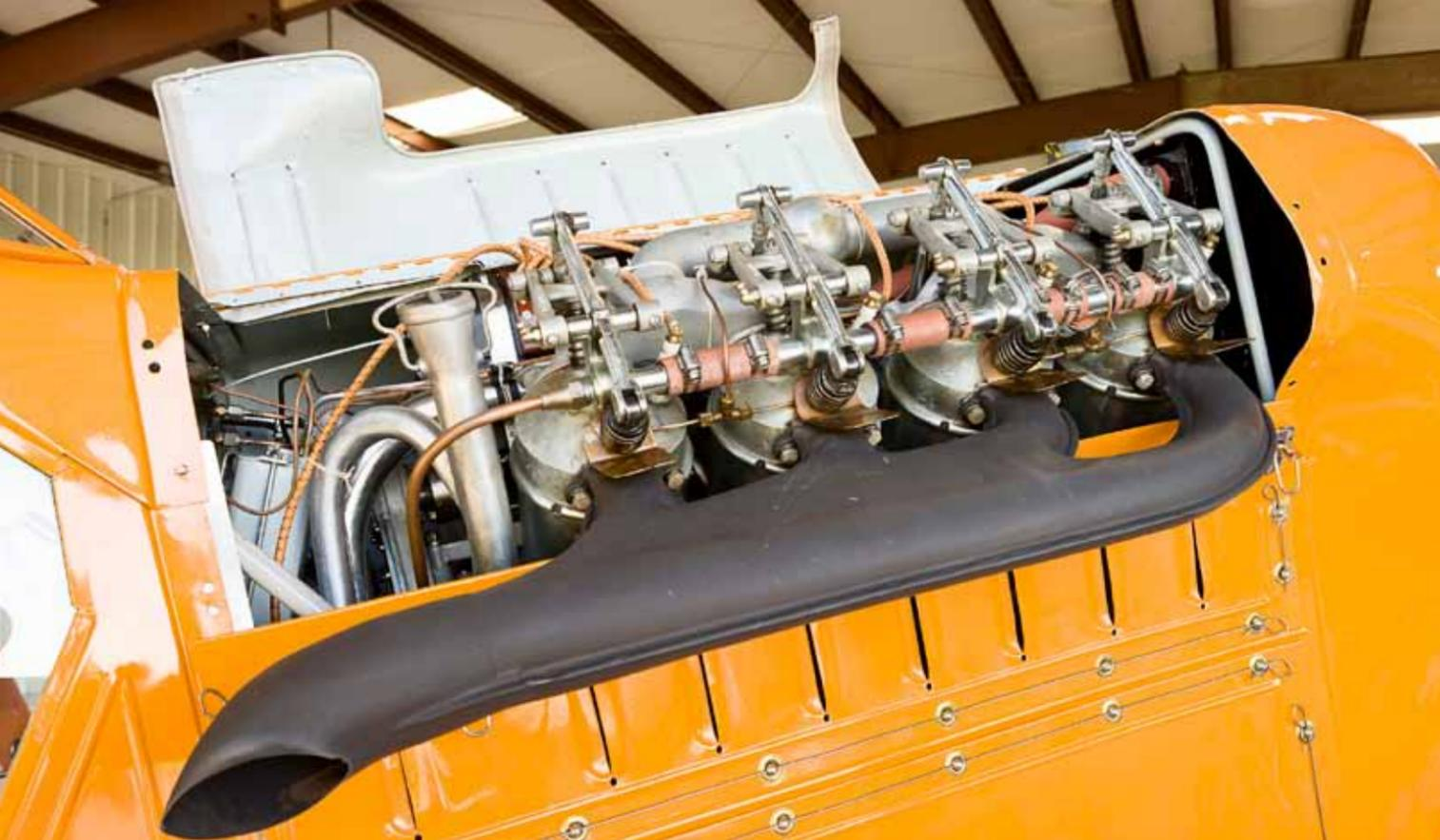
The water-cooled Curtiss OX-5 V-8 engine (left) does not have rocker (valve) covers to protect rocker arms, valve stems, and valve springs. The instrument cluster (below right) contains the altimeter, tachometer, oil-pressure gauge, and water-temperature gauge. The airspeed indicator is above the cluster.
